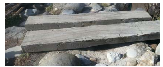
SHOTCRETE LOGS PRECEDENT IMAGE
